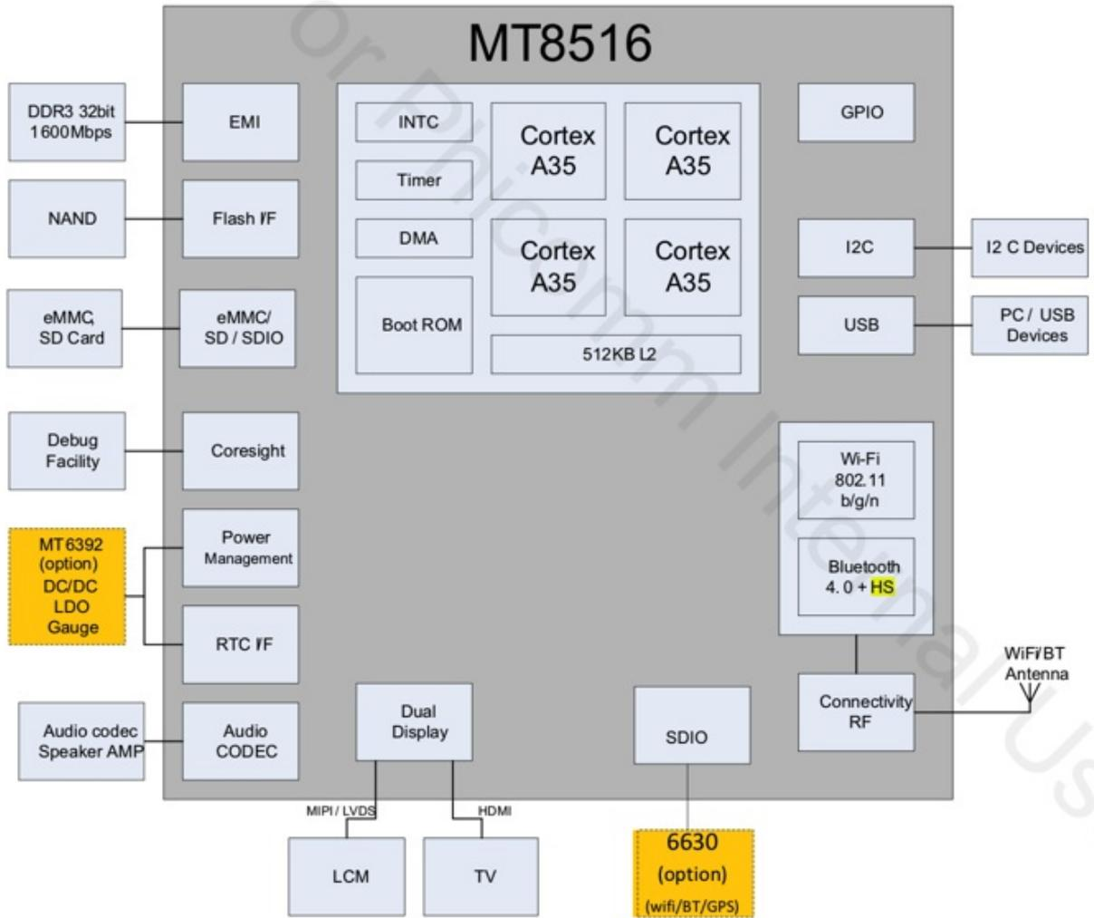
**Figure 1-1: MT8516 Block Diagram**
