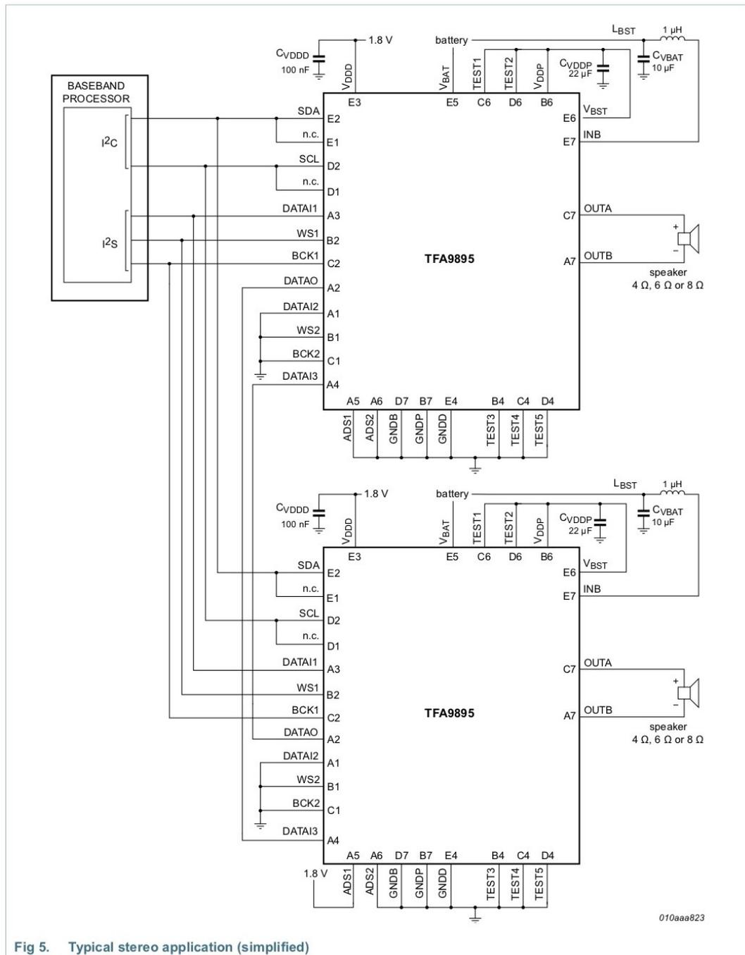
Fig 5. Typical stereo application (simplified)
